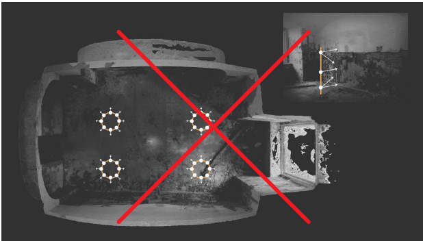
Fig. 4. An incorrect method of selecting locations for making images
